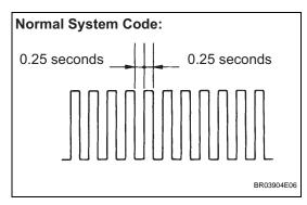
(c) Check that the warning light blinks in a normal system indication pattern.
