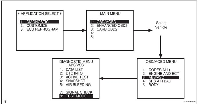
Switch the ECU to test mode using the intelligent tester.
